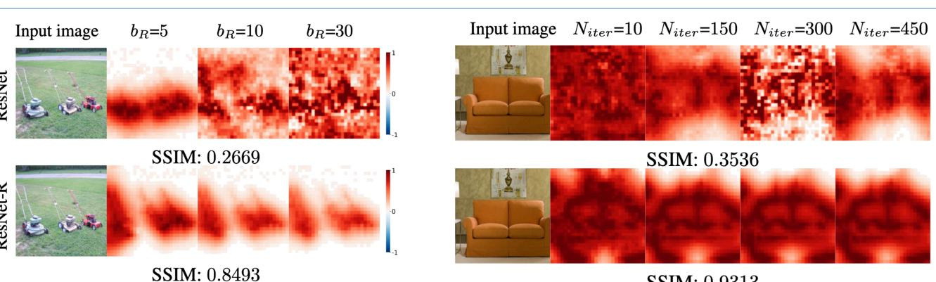
Meaningful Perturbation (MP) heatmaps for ResNet vary dramatically. In contrast, MP heatmaps for robust models (ResNet-R) are ~1.4 × more consistent under SSIM metric and converge faster (10 steps vs. 300 default).
